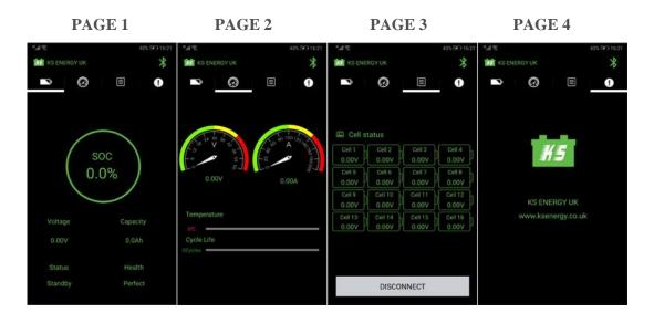
The battery information within the application is essentially self-explanatory and an overview follows: Page 1 displays State of Charge (SOC) as a percentage, the battery Voltage, total Capacity, and the present Status
